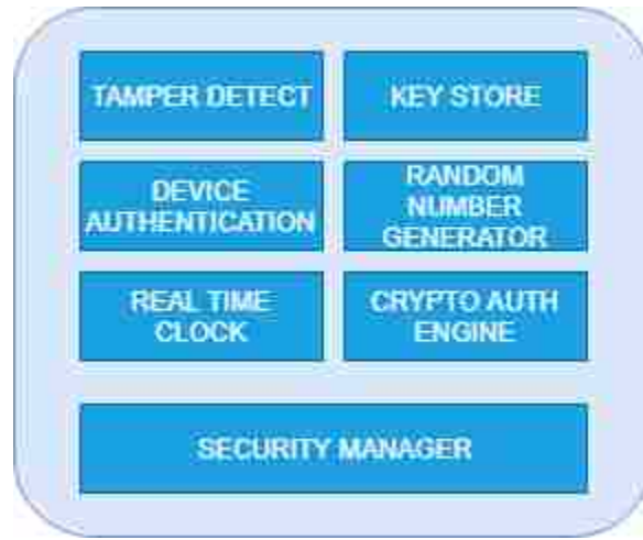
Figure 5.3: TPM Block diagram
